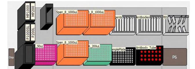
Figure 5: (Right) Biomek 4000 Deck Layout houses all samples, tools, tips, and reagents simultaneously.
